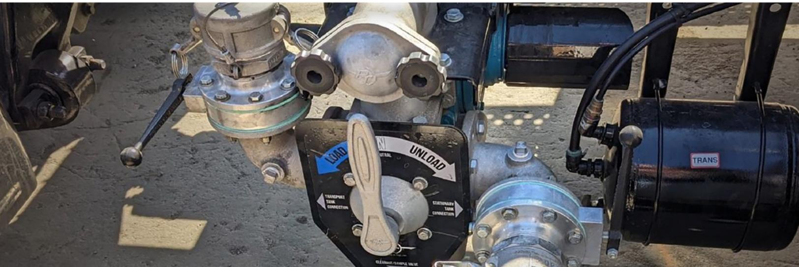
PT's **FCS-V3N VANE SYSTEM** (Item No. 100414), is a 72 lb. (without pump) assembly that is designed for loading and unloading refined fuels utilizing a 3" vane pump. While the FCS-V3N system is truck mounted on the driver's side or curb side, the system is available with a crossover kit that allows for trans-loading from the opposite rail.
